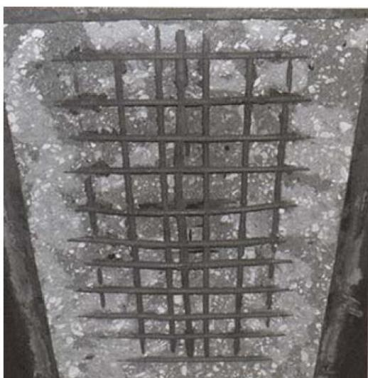
a) without fibre reinforcement
